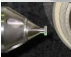
NC cylindrical grinding: Machining a small-diameter grinding wheel using an index device
